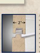
A **Full Thermal Break** is used in the tongue-andgroove construction of all 2000 series doors. This rigid vinyl extrusion seals the joints and eliminates metal-to-metal contact, which limits the transfer of temperature.
